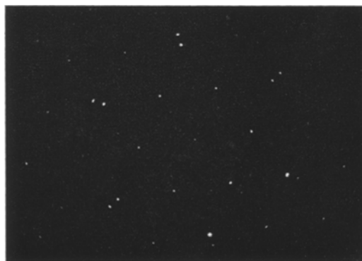
Figure 6 SAED of a \text{Co}(\text{OH})_2 particle at the beginning of oxidation in an air flow at room temperature.
