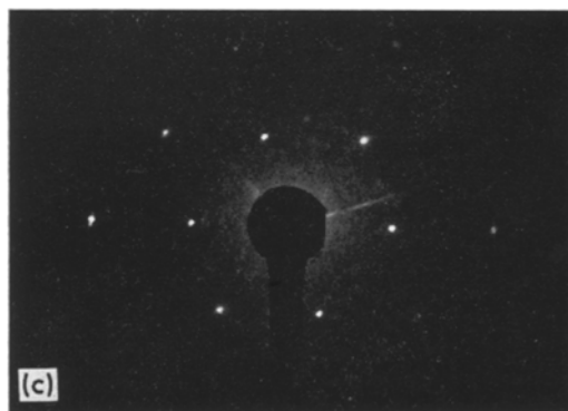
Figure 8 (a) Cluster of \text{CoOOH} flakes obtained by oxidation of \text{Co(OH)}_2 in hydrothermal conditions. (b) SAED of the same cluster: pattern of a single crystal lying on the (0001) plane with central extra spots. (c) SAED after 36^\circ tilting around an axis of the (0001) plane.
